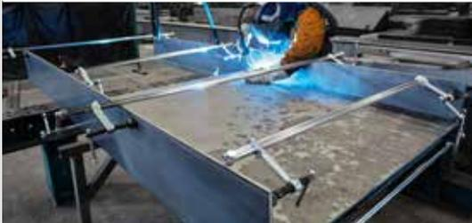
Alongside complete assembled high-performance clamping sets BESSEY also offers versatile accessories that can be combined with one another. Sliding arms that are already fitted can be changed over from clamping to spreading or replaced by different sliding arms or even supplemented with others.
