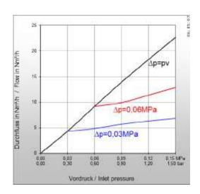
\* Conversion factor 2.5 for devices comprising a flame arrestor The conversion factor for free flow is 3.8 ( Reference: BAM report 220, D .Lietze) Example:
